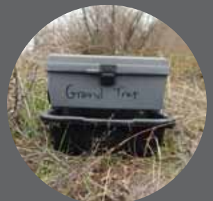
Gravid Trap for egg-carrying mosquito surveillance
