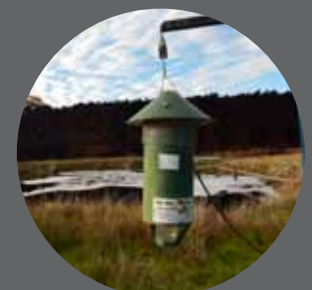
New Jersey Light Trap for mosquito population surveillance
