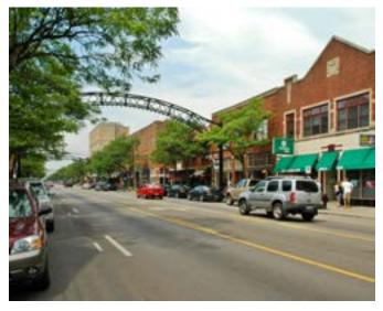
Figure 3.10. Gateway treatments may include parking, lane narrowing, street trees, medians, lighting and monuments. *Source: Toole Design Group*
