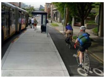
Figure 2.12. Separated bike lanes are located adjacent to a bus stop on this Seattle roadway. **Source: Humantransit.org**
